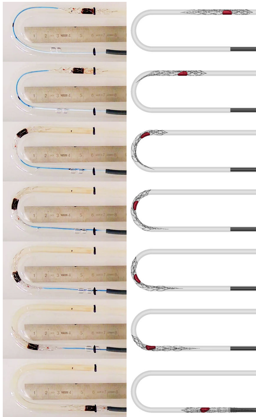
Figure 5. Comparison between the in vitro (left panel) and the in silico (right panel) thrombectomy test in the glass U-bent vessel. In both the results the clot, trapped in the stent, is successfully retrieved until reaching the aspiration catheter.
